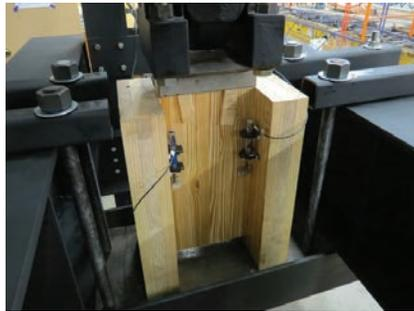
CLT studies at Clemson University's Wood Utilization + Design Institute in Clemson, S.C., include testing the performance of structural adhesive between the flanges and the web of a specimen. Image courtesy of Clemson University, Wood Utilization + Design Institute
