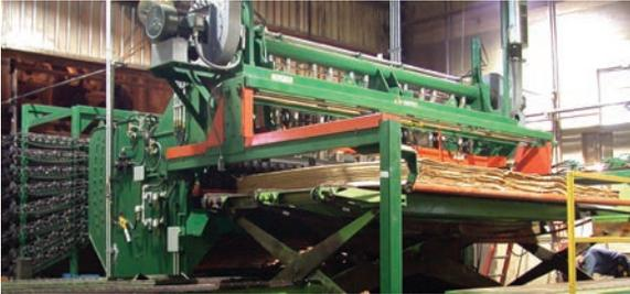
The Sweed **Accumatic** eliminates time loss in the veneer drying process caused by charge breaks.
