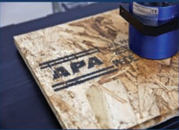
REA JET DOD Marking on OSB Panels
