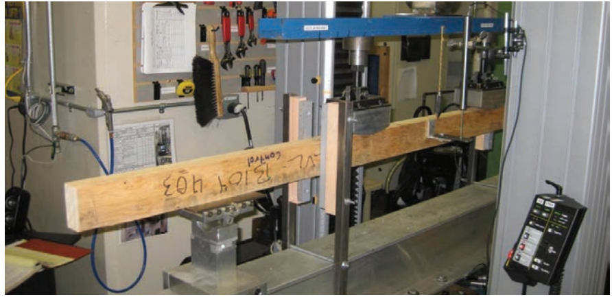
A thermally-modified LVL specimen undergoes bending strength testing.
