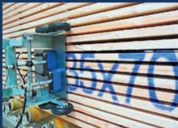
REA JET DOD Marking on Timber Board Stacks
