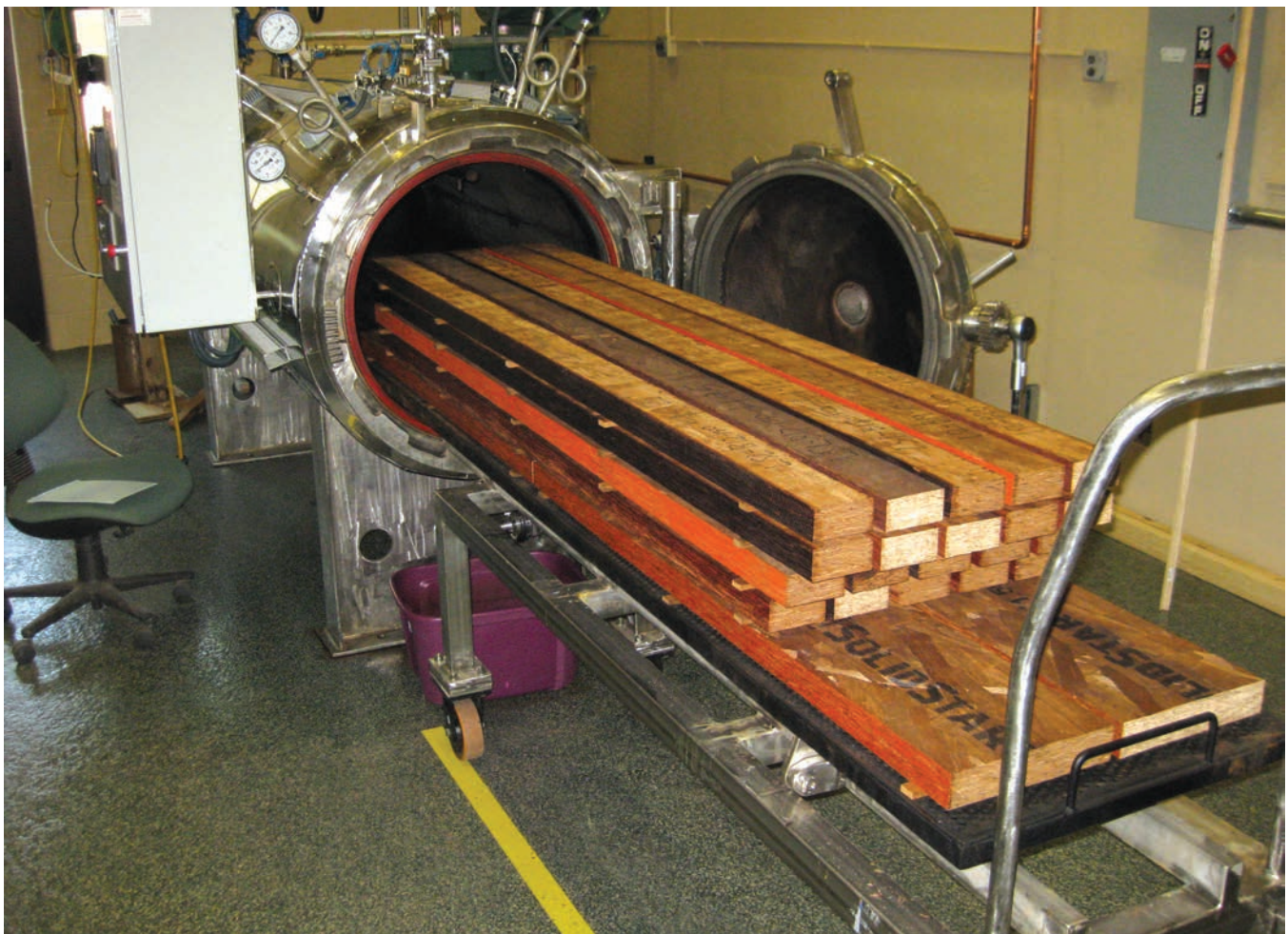
Laminated strand lumber (LSL) is removed from the thermal-modification kiln after treatment.
