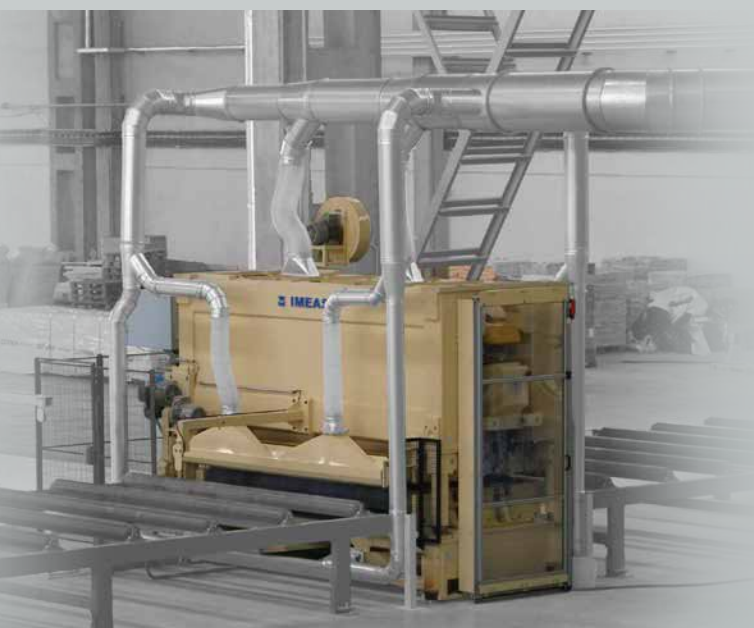
IMEAS 12' wide Cross-Laminated-Timber (CLT) Sanding Line
