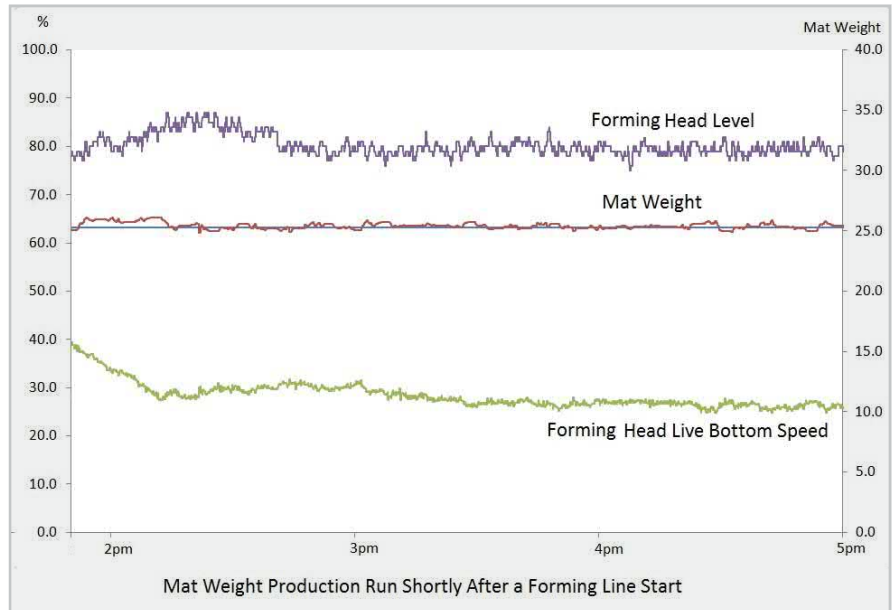
This graph shows how mat weight is stabilized using the Smith Predictor algorithm.
