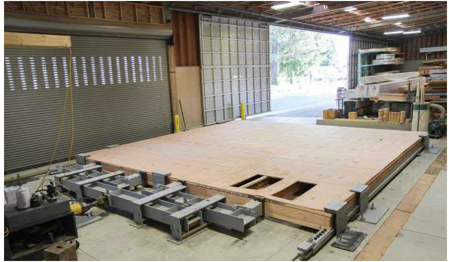
Lack of space in APA’s existing lab necessitated construction of an addition adjacent to the lab in 2006 to test even conventional 24-ft-by-24-ft diaphragms. The main lab’s new, column-free space will allow for larger configurations as well as U- and L-shaped assemblies.
