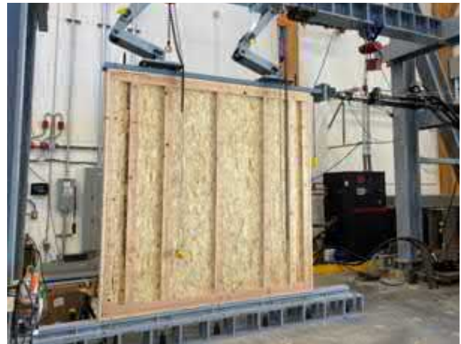
Figure 2. A high-strength shear wall test is conducted at the new APA laboratory.
