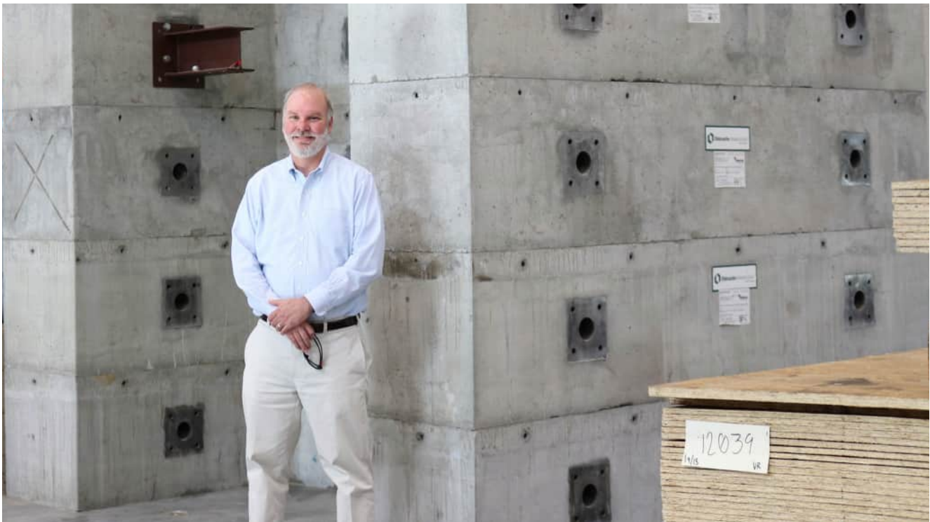
APA's expanded research center includes concrete block strong walls with anchors and a 4-foot-thick reinforced strong floor to accommodate full-scale multi-story structural assembly testing.
