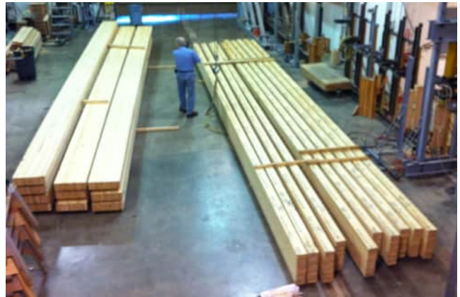
2011-2015: A portion of the glulam beams used for the full-scale in-grade glulam tests validates current glulam design values.
