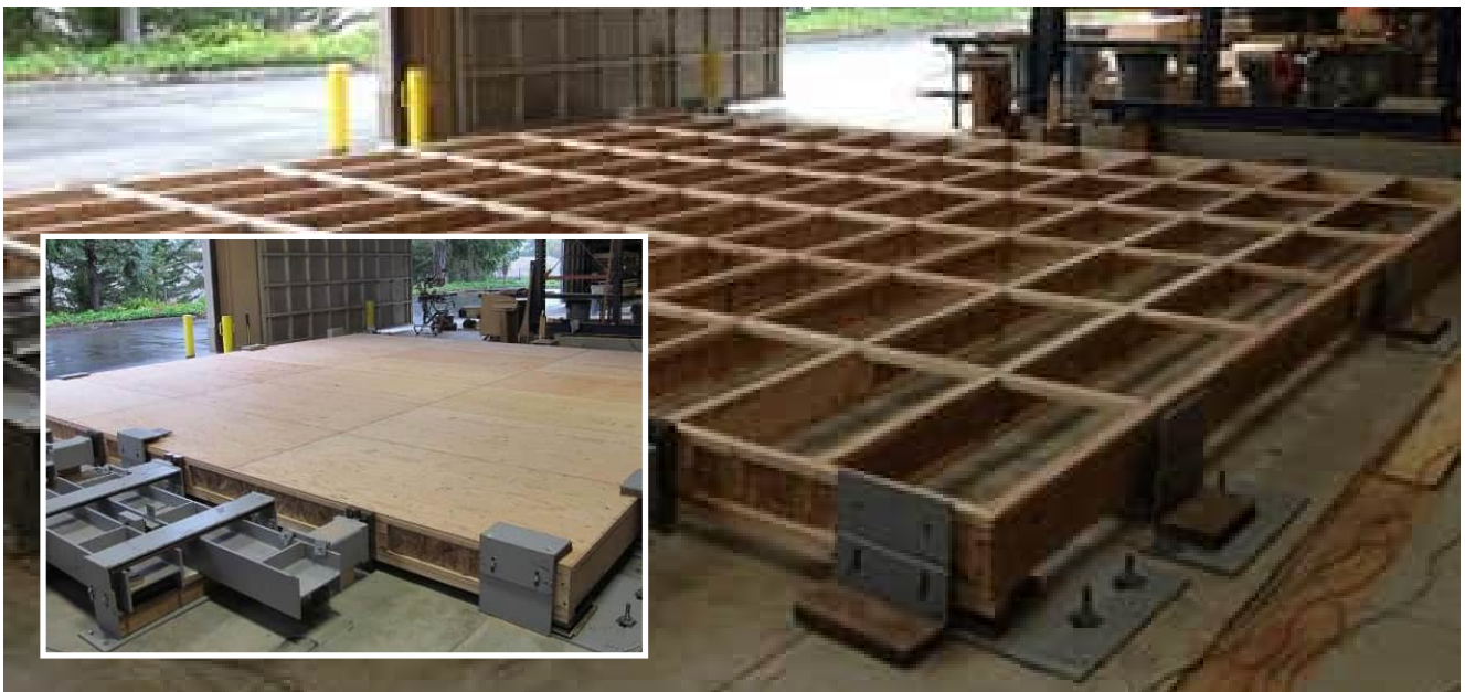
2016: Testing of a full-scale (24-foot by 24-foot) diaphragm using I-joint framing to establish diaphragm design values in light-frame wood construction.
