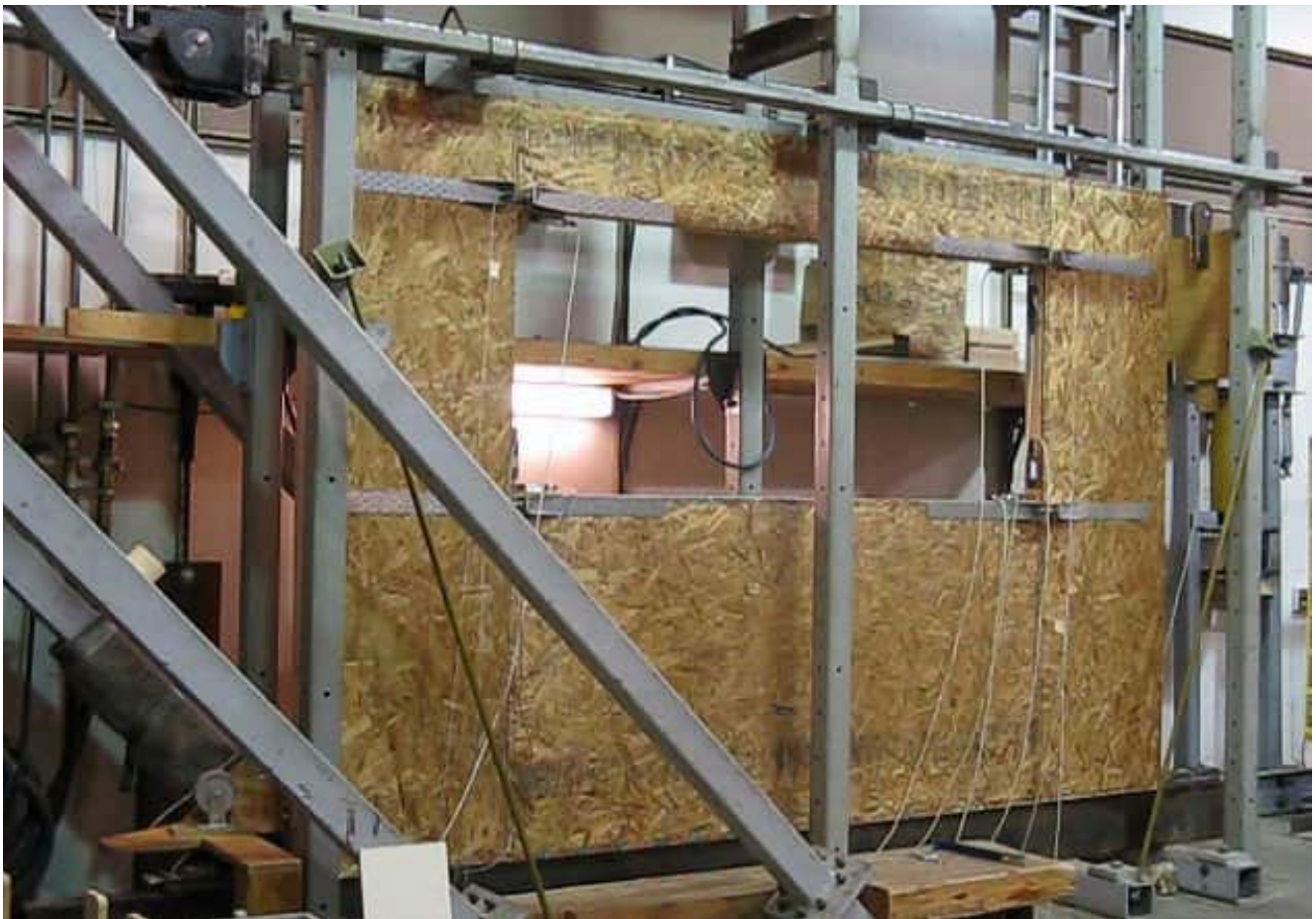
2009-2010: A full-scale shear wall test supports the use of wood structural panels with a large wall opening.
