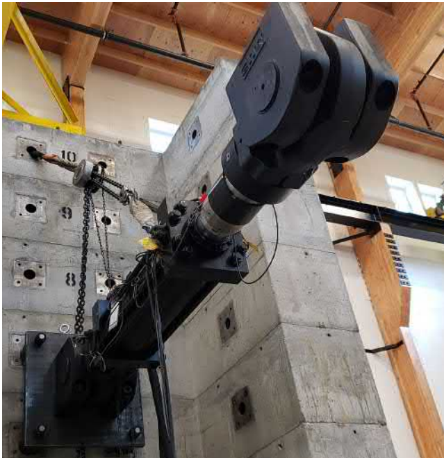
20-ft tall stackable strong wall and a 220,000-lbf actuator
