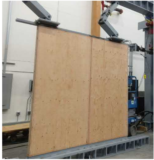
Full-scale shear wall test frame with strong arms
