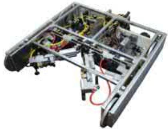
KTC solution: a high temperature OSB Press Repair Robot capable of repairing press dents by welding and grinding.
