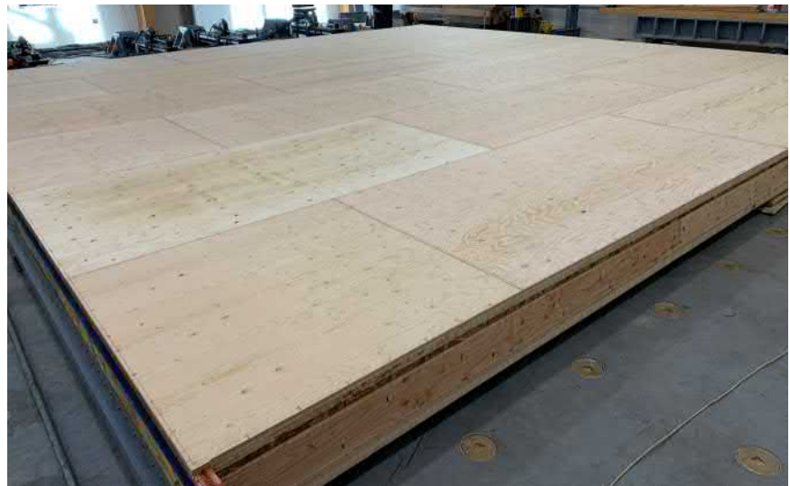
24 ft by 24 ft full-scale diaphragm test setup
