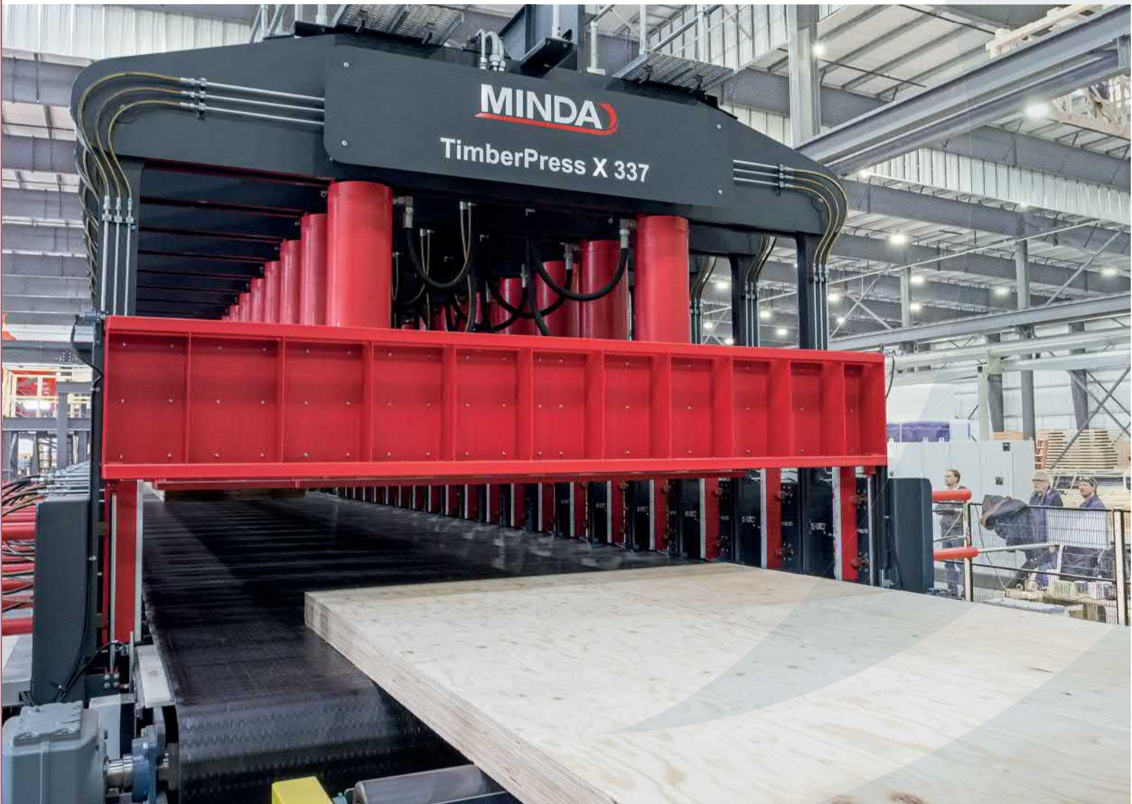
cross laminated timber press: TimberPress X 300
