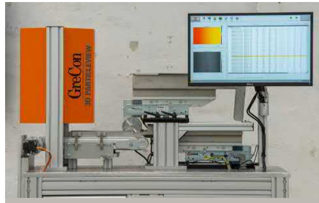
Fagus GreCon: 3D ParticleView measuring unit that assesses wood particle quality.
