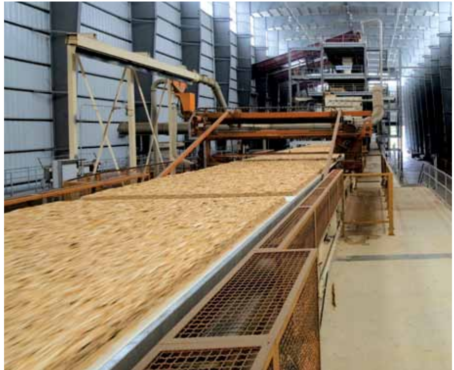
This cross-cut saw in RoyOMartin's OSB mill in Oakdale, La. cuts mats to various lengths.
