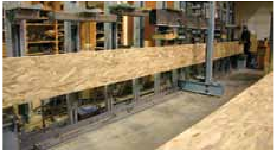
APA full-scale bending test equipment tests glulam, I-joist, and structural composite lumber.
