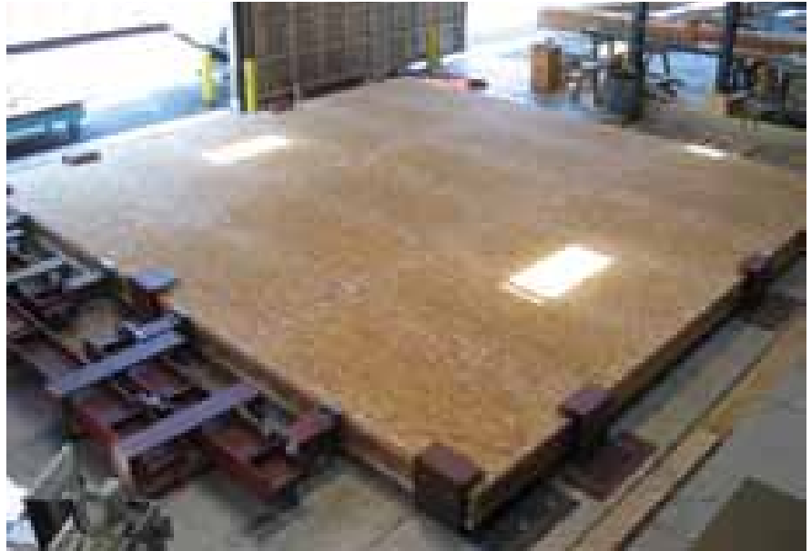
APA full-scale (24-ft x 24-ft) diaphragm test equipment is shown at the APA Research Center.
