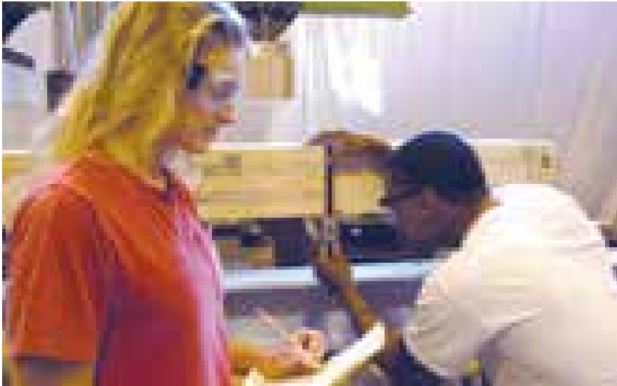
Undergraduate student researchers Catherine Juca and Anthony Holliman test the strength of a cross-laminated timber beam on a 50,000-lb capacity materials testing systems machine in the Department of Sustainable Biomaterials, College of Natural Resources, at Virginia Tech.
