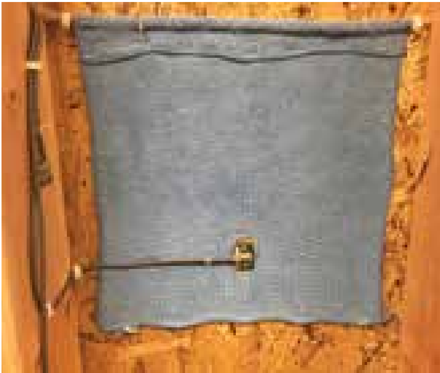
The "wetting apparatus" applies water to a towel that is placed over the inside surface of a wood structure panel. The simulated water leaks will test the wall assemblies' ability to dry out the excess amount of moisture.
